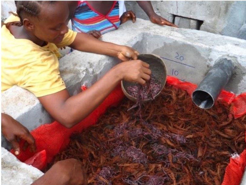
Picture 8: Provision of worms to the biodigester.
